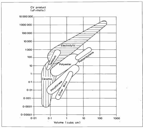
Figure 2. CV product and volume of capacitor range.
