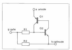
Figure 1. 2 transistor equivalent of a Thyristor
