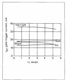
Figure 5. Peak gate trigger current as a function of trigger pulse duration
