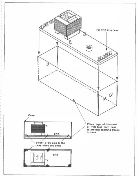
Figure 5. Mounting Module into Case.
