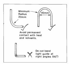
Figure 13. Bending the Light Guide.
