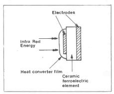
Figure 1. Pyroelectric Element.
