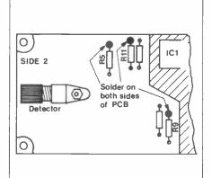
Figure 11. Some resistors are soldered both sides.
