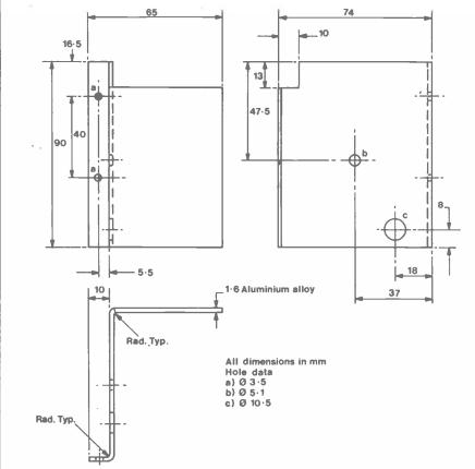
Figure 12. Transformer Bracket.
