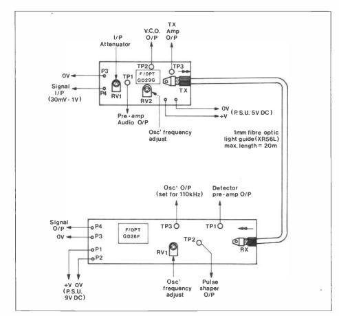
Figure 12. Connecting up the System.
