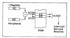
Figure 4. The Z80 Mode 2 interrupts.
