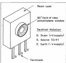
Figure 6. Sensor pin-outs.
