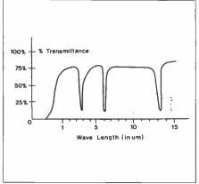
Figure 10. Window Spectral response.
