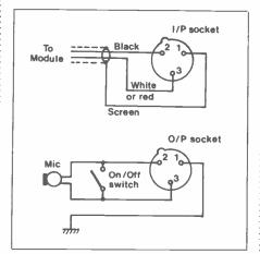
Figure 7. Wiring XLR Connectors.
