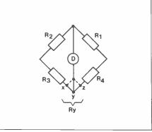
Figure 2. Measuring Resistor Values below  $1\Omega$ .
