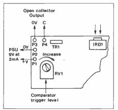
Figure 9. External PCB Connections.
