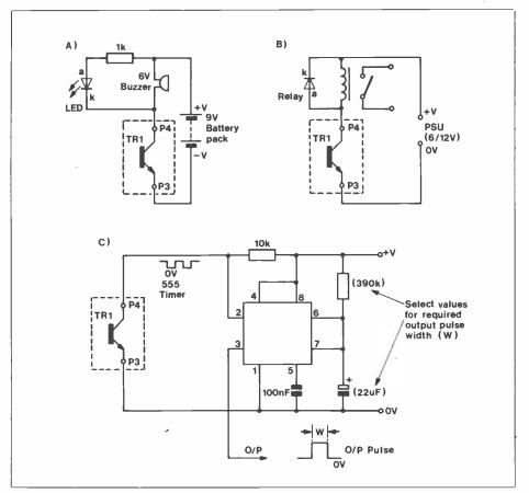
Figure 8. External Circuit Connections.
