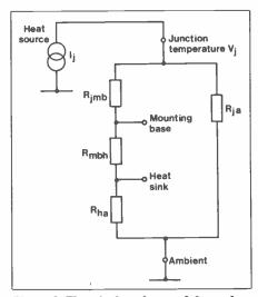
Figure 8. Electrical analogue of thermal circuit
