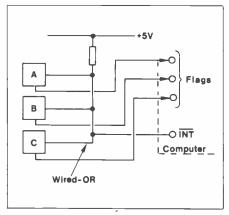
Figure 2. Three peripherals A, B and C connected to a common interrupted line.
