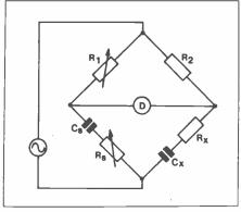
Figure 8. Bridge for Measuring Capacitance.
