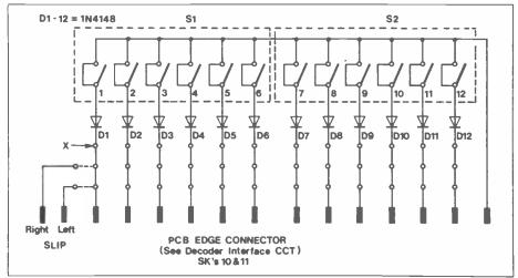
Figure 4. Diode Card Circuit.
