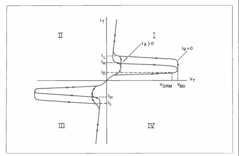
Figure 4. Dynamic main current/main voltage characteristics
