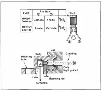
Figure 2. Emitter and Detector Pin-out and Construction.
