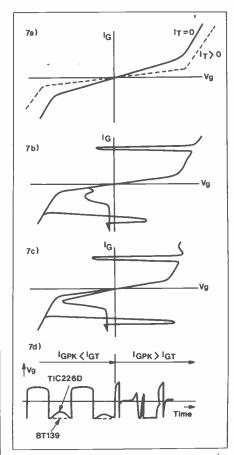
Figure 7 (a). Gate dynamic characteristics with gate and main currents in phase.
