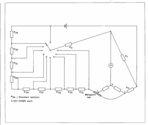
Figure 4. Stepped Resistors.
