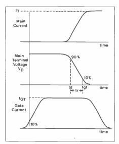
Figure 6. Timing diagram for the triggering process
