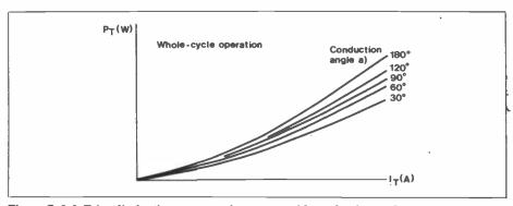
Figure A. 2. 1. Triac dissipation verses main current, with conduction angle as parameter.
