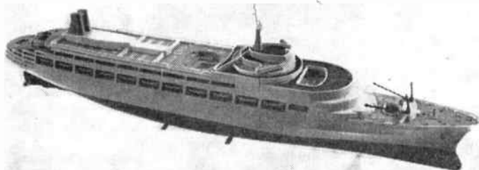
The first passenger liner in the Airfix range is the Canberra the kit for which has 86 detailed parts and costs 7s. 6d. The finished model is 16 \frac{1}{2} in. long and is to a constant scale of 50 ft.:1 in. Modellers will appreciate the faithful reproduction of many unusual features in this ship.
