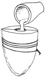
Fig. 2-Mould being poured
