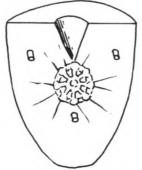
Fig. 1—The two halves of cuttlebone mould showing pour, impression, locating pins and scratches to release air
