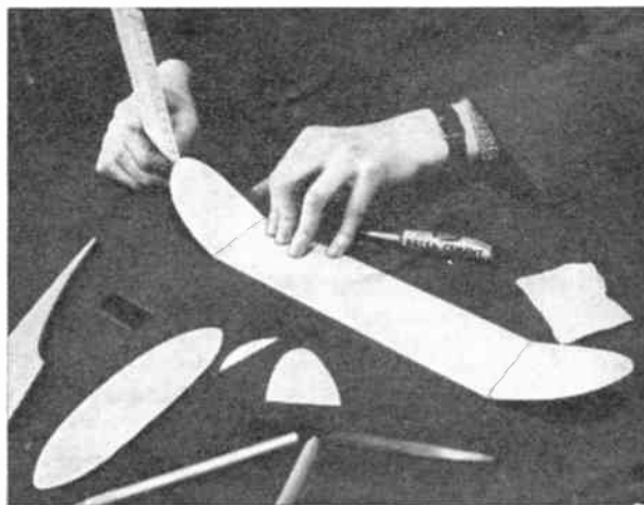
Checking dihedral on wing tips
