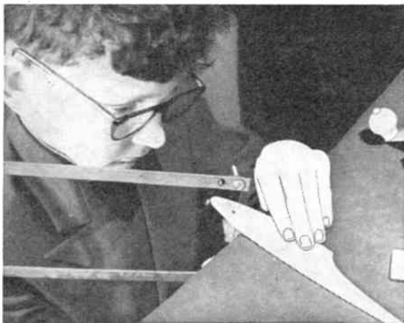
Cutting hole in nose for ballast
