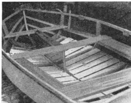
The hull completed for sailing, with the centreboard fitted in its case and side benches between the thwarts
