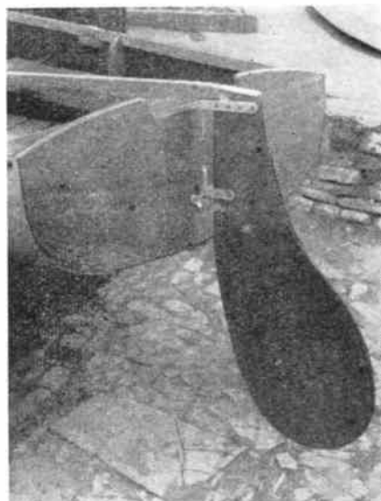
The rudder in position on the transom
