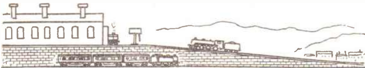
A GOOD WAY TO BRING IN DIFFERENCE OF LEVEL - A RAISED LOCO DEPOT.
