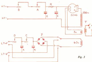
The electrolytics (K,K) shown in the diagram were 1,000+2,000 types. They were connected together at the bottom of each can for the negative pole. The 1,000 mfds. tags of both cans were joined to form a 2,000 mfds. first positive pole, while the 2,000 mfds. tags were treated similarly to produce a 4,000 mfds. second positive pole. This latter is joined to the left outer tag of variable resistor (C), as shown.
