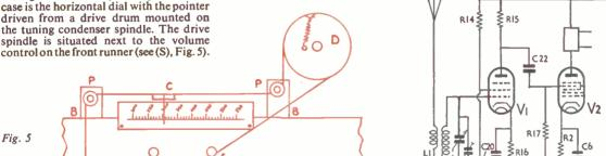
The size of the drive drum (D) will depend on the size of the dial. Its radius will be the length of the scale divided by 34. Dials can be bought, and for a cheap yet attractive one I recommend the 'Superex' dial (at 2/6) from Superior Radio, 37 Hillside, Stonebridge, London, N.W.10
