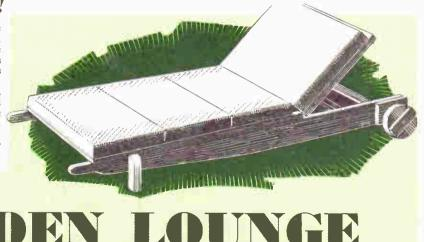
The wheel ends are simply rounded at one corner and the other ends tapered off to form handles. These should be rounded slightly on the undersides.
