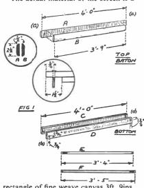
rectangle of fine weave canvas 3ft. 9ins. by 3ft. 2ins. This is first given a coat (or two if necessary to cover well) of flat white paint. When dry, this base is followed by two coats of aluminium paint. Rather more than a quarter pint of this will do the job well. Finally, put on a dark blue border as Fig. 3. This is lin. wide and at the sides. Top and bottom are not painted blue as the battens complete the edging here.
