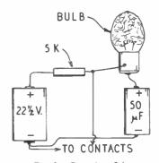
Fig. 3—Capacitor firing
