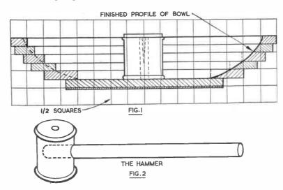
The bowl is now ready for the anvil which is made from an empty cotton reel. Plug the centre hole with a piece of dowelling and glasspaper the ends flush. Glue the anvil into place, at the bottom of the bowl at the centre. The whole may be finished by staining and french polishing, or if made of two contrasting woods french polish only with clear shellac.
