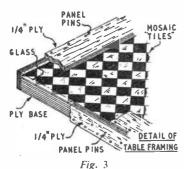
Another method to finish the top is to apply squares of contrasting wood veneer, as used in marquetry. These are glued in place with cellulose cement glasspapered flat and smooth and either wax polished or varnished. Ordinary framing is fitted.
