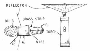
Fig. 2-Open flash unit for torch
