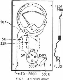
With a 0-5mA meter voltage ranges to suit can be chosen, such as 0-5 V and 0-50 V, etc. If this is done, the meter scale can be left unchanged, and readings will still be easy.
