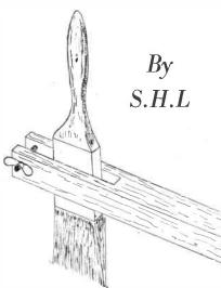
THERE are times when one wishes the paint brush had a longer handle or could be made to extend a little further to avoid moving the ladder so many times. This applies
