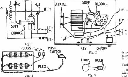
For condenser 'C' an air-spaced preset condenser is best, and these can be obtained quite easily. The value of this type is about 30pF, but a condenser of between 25pF and 50pF can be used. A tag strip is also necessary to support the aerial coupling coil ends and connections, and a 2-way socket (or pair of output as the 3D6. They may, however, deliver enough power, according to the maximum range wanted.
