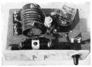
One-valve model control transmitter
