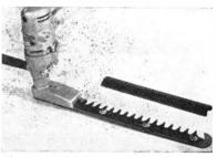
The new Black & Decker Hedge Trimmer and Pruner attachment, shown here powered by the  $\frac{1}{2}$  in. Sander Polisher Drill. The slip-on blade guard converts the attachment for pruning.
