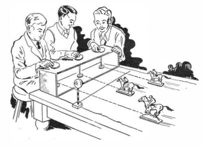
The wheels should not scrape when turned and some adjustment may be necessary here. Also the handles should be free to turn on their screws. The box should be glasspapered smooth, and painted a bright colour. A name for each horse can be lettered in black on a strip of card, and this glued along the top front edge of the box.
