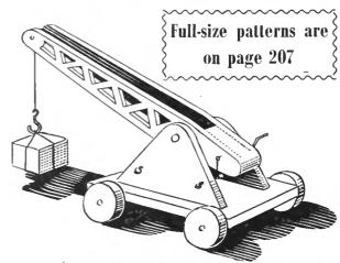
The wheels (F) are but from \$\frac{1}{4}\$in. wood and attached to the axles (C). A small piece of round rod pivots the crane arm, and pieces of wire are bent to form the handles. The cord passes over a fretpin which is pushed through the top of the
