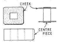
Fig. 2—The bobbin to hold the windings
