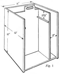
glasspaper the opening quite smooth to make a comfortable grip for the fingers. Join the two divisions together, then fit inside the box and firmly nail therein. Add two or three thin screws, driven through the bottom of the box into the 'handle' division. The bottom of the box should not be nailed on, but cut to fit
