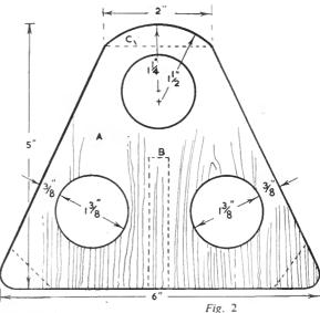
Transfer the patterns you have now completed to suitable wood, using a piece of carbon paper in the usual way. The base will be \(\frac{1}{2}\)in. thick, and the handle \(\frac{1}{2}\)in. Let the grain run in the direction shown by the diagrams. Utilize a straight edge of your wood where possible to save cutting.
