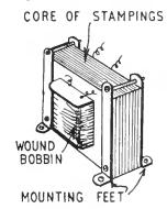
Fig. 3—A completed transformer
