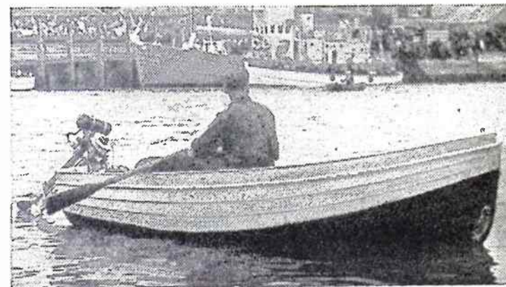
A typical clinker built dinghy—not so easy for amateur construction, and generally avoided in favour of ply skinning
