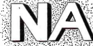
Fig. 5—An appearance of relief can be secured by shading the sides of an article further from the light source
