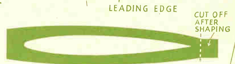
ENGINE NACELLE E. CUT TWO 3/16in. ENGINE NACELLE F. CUT TWO 3/8in. GLUE TOGETHER ONE E AND ONE F.
