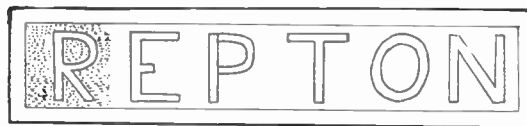
Marking out the board. The dotted surface shows where the matting punch is used on the background
