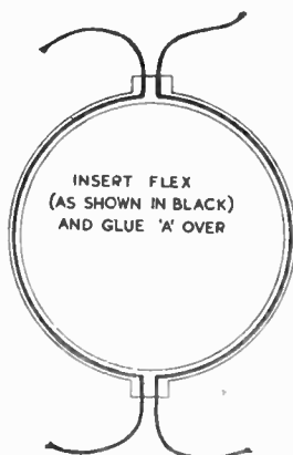
Fig. 3—Flex in place
