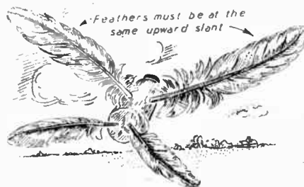
Fig. 6—A simple feather giro glider
