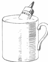
Stand the tube in warm water to soften
