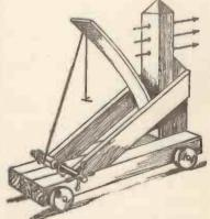
spears in the holes drilled for them (they must fit loosely in the holes), then pull the trigger cord and release the striker, which will drive the spears forward.
