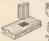
Fig. 1.—The Base with hole cut to take the upright.
