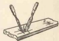
Fig. 8.—How to cut the Mortise.
