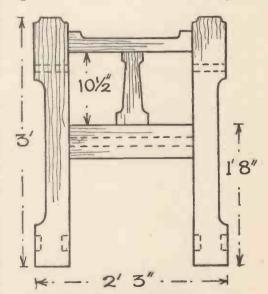
Fig. 1.—An Elevation of the back of the Chair, with useful Dimensions.
