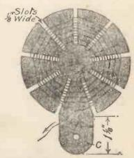
Fig. 2.-How the Basket Coils are made.
