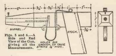
OU will require some 1-inch square wood, 12 in. long, an old clock spring about \{\frac{1}{2}} in, wide, and a pin to make this simple and cheap gun. The bullets are ordinary matchsticks, and can be fired a considerable distance. You will notice that the gun consists of two main parts; they are called the stock or handle, and the barrel or tube through which the matchsticks are fired.
