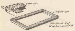
Fig. 3.—The Chase in which the Type is held or Set.
