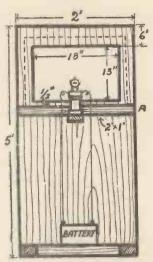
Fig. 3.— The Measurements for cutting the Stage Opening.
