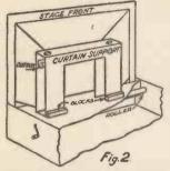
How the Curtain Support is fixed to the Stage
