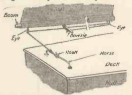
Fig. 1.—The Main Sail must swing from side to side to an extent governed by the cord called the Main Sheet.
