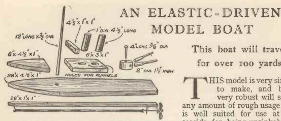
Fig. 2.—The Component Parts of the Battleship.
