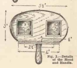
thin edges facing each other. Glue narrow strips of wood round the lenses to keep them in place, and remember that the lenses should be flat at the eye side, which will mean that, owing to their wedge-shape, they will be at an angle on the view side.
