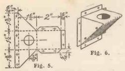
Figs. 5 and 6 .- How to mark out and assemble the Chimney Support.
