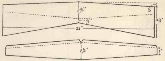
Figs. 3 and 4.—Details of the Wings.
