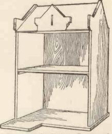
A Picture of the Skeleton Framework without the Door, to show the General Construction.
