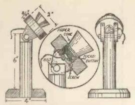
Fig. 5.—The Stand for the Microphone.
