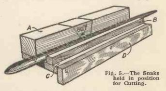
block like this. The two kerfs, or saw-cuts, are at 60 degrees to the top of the block and are used to guide the saw when cutting the snake. A strip of wood (B) is fastened on the bottom board, C to hold the snake secure, and the strip marked D is gripped in a vice. When sawing out the wedges of wood take particular care to avoid quite reaching the tape.
