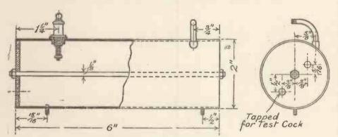
Fig. 3.—How the Boiler is made.
