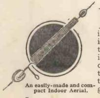
ROCURE about 30 ft. of bare copper wire, and wind it closely round a broom handle; now slide it off the stick and twist one end into a loop, as shown in the sketch. Attach two insulators of the egg type to each end, and stretch the coiled wire out to the required length, fixing it by means of cord to the wall. The lead-in can next be soldered to the loop in the wire, and then carried down to the set. Although not extremely efficient, this aerial will give results on a good set.
