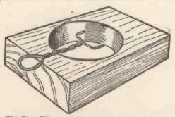
Fig. 4.—The mould for the lead weight.
