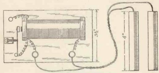
Fig. 1 .- Plan View of the Shocking Coil.
