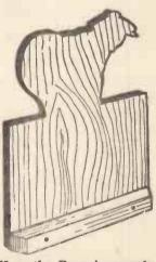
a strip of wood glued and nailed along the back.
