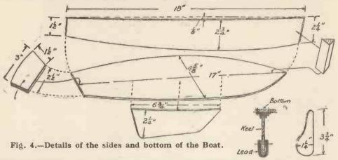
The Transom.—The stern piece, or transom (Fig. 4), should be made of thicker stuff than the rest of the hull—say  $\frac{5}{16}$  in thickness wood of close grain—and be very slightly carved on the top line. The stern end of the sides will require planing at an angle so that they meet without a gap when fixed up
