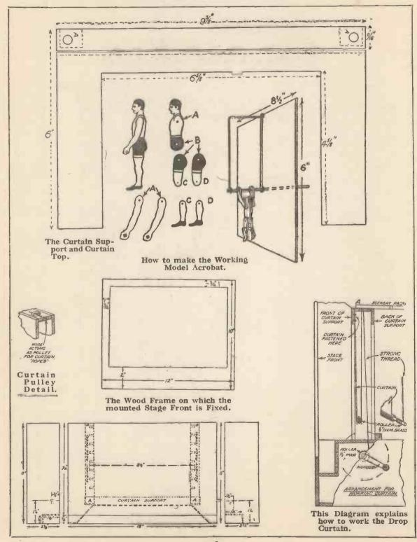
wings. Some constructors may have some small pieces of wood available which could be used up by mounting them separately. The overall dimensions of each one is 6 in. long by about 13 in. wide. The slots in the scenery racks will take wood up to a thickness of  $\frac{3}{16}$  in. Now cut the exterior wings out, but do not cut
