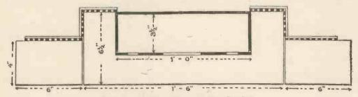
Fig. 2.-A Plan View of the Station.
