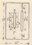
Fig. 5—The Top of the Box, showing the Position of the Dog and Money Slot.
