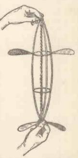
Fig. 8.—How to launch the Model Helicopter.
