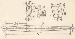
Fig. 3.—The Jib Winding Handle and Brackets for the Wheels.
