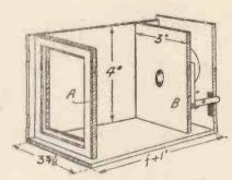
Fig. 2.—Details for fixing the Lens Board.
