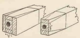
Figs. 3 and 4.—How to Shape the Front of the Barrel.
