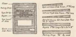
Fig. 4.—How the Type is Set in the Forme.
