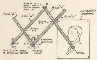
Fig. 1.—The Pantagraph completed. The assembling of the Parts is shown in this Diagram.
