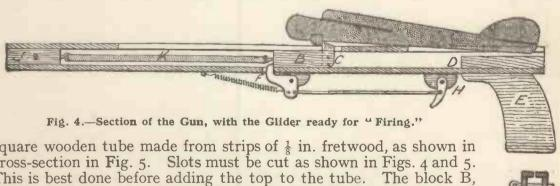
square wooden tube made from strips of \( \frac{1}{8} \) in. fretwood, as shown in cross-section in Fig. 5. Slots must be cut as shown in Figs. 4 and 5. This is best done before adding the top to the tube. The block B, then, may be made and fitted so as to run freely through the tube. At its back end a saw-cut is made, into which the brass strip C is inserted and secured with two rivets. The projecting head of the strip must have a free run along the slot (see Fig. 4). At the
