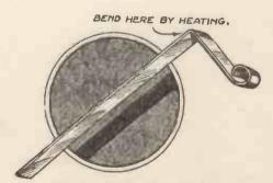
Fig. 7 .- The Firing Spring.
