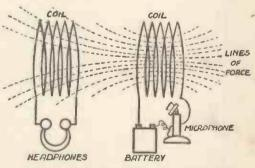
Fig. 1.—The Principle on which the Telephone works.
