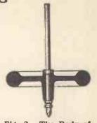
Fig. 2.—The Body of the Top can be made from a single Brass Casting.
