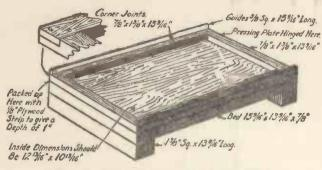
Fig. 1.—How to make the Press Bed.
