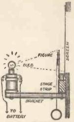
Fig. 5. -The Lighting Arrangement.
