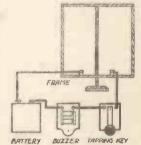
Fig. 6.—Substituting a Buzzer and Tapping Key for the Microphone.
