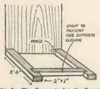
Fig. 2.—The Supports for the Front.
