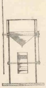
The Hopper and Sandwheel Mechanism.
