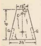
Fig. 2 .- The Measurements of the Side Pieces, marked C C in the Finished Model.
