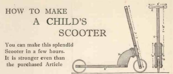
Fig. 1.-A Side and Front Elevation of the Scooter.
