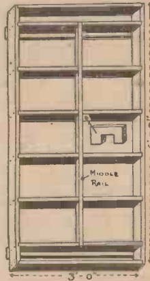
Fig. 1.—The frame for a 6ft. 4in. table.
