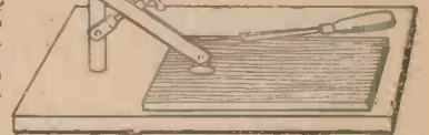
Fig. 2.—Above, the work is fixed with two light steel cramps. Another method shown is to use Hobbies' Bench Cramp on the wood.
