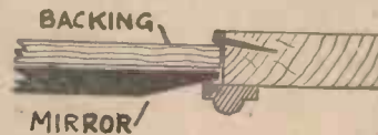
Fig. 5.—A section to show how the mirror is fixed in. Notice the backing held by a "sprig" or nail.
