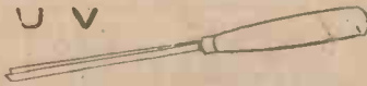
Fig. 3.—The U and V are the shape of the most common chisels needed.
