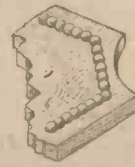
Fig. 3.—A "close-up" of the beading to show the joint at the corners.
