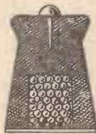
Fig. 2.—How the chessmen are weighted.
