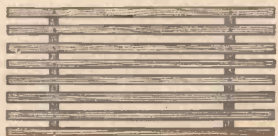
Fig. 2.—The grating for the bottom of the punt. (Continued on page 834.)
