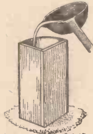
Fig. 3.—Moulding the lead weight.
