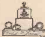
Fig. 11.—The bridge which carries the screw to adjust the tension of the armature.
