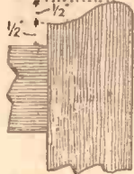
Fig. 2.—The shape of the rail ends, and the position of the cross rail.
