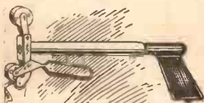
The "pop" from this gun is provided by the bursting of a film of paper.
