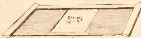
Fig. 4.—Another view of the back showing three of the outer rails in place on the large board which forms the back.
