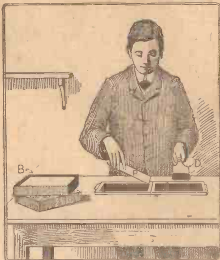
FIG. 2.—METHOD OF INSERTING A DRY PLATE IN THE DARK-SLIDE OF CAMERA.
