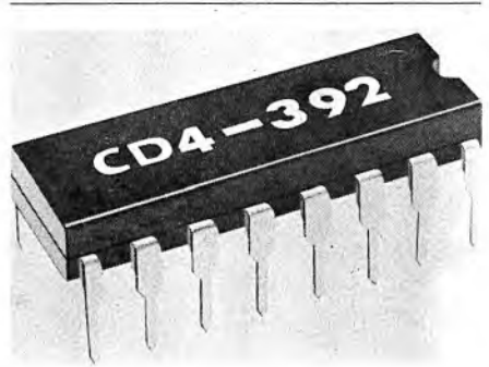
Signetics/JVC CD-4 demodulator chip features automatic carrier level adjustment to cater for various pickups.
