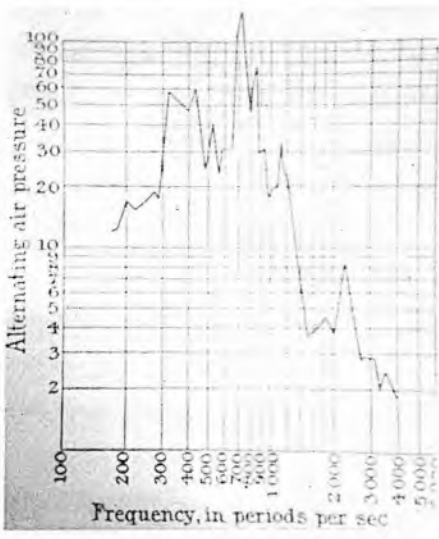
Fig 11 Considered as a typical frequency for a loudspeaker in the 1920s. Note the amplitude scale in 'alternating air pressure' instead of the now more familiar dBs.
