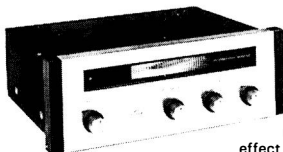
SX-440 AM/FM Multiplex Stereo Receiver Music power output: 40 W at 4 ohms (IHF) Frequency response: 20 to 70,000 Hz \pm 3dB (Overall) FM Frequency range: 87 to 108 MHz.
