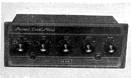
Leak point one plus control unit
