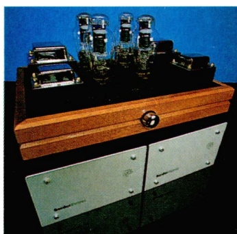
The P20 power amplifier, with exposed valves, transformers and optional volume control, sits atop its twin power supplies.
