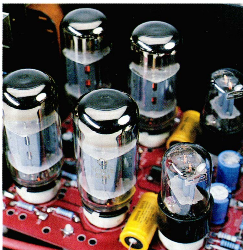
The P2SE amp uses pentode output valves in parallel single ended operation.
