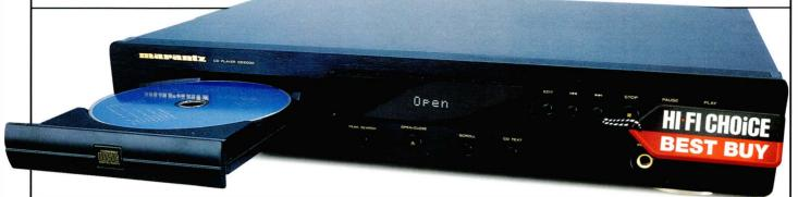
he CD6000, the base version of the 6000 OSE reviewed previously, is a one-bit player, with bitstream converters that are driven in dual differential mode to improve linearity and reduce noise and distortion. An HDAM buffer amplifier is included to ensure low output impedance, and a high slew rate output. The disc drive mechanism is the VAM 1201, a floating design, used with a digital servo.
