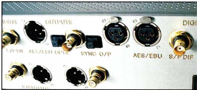
The Chord's back panel is equipped for every digital eventuality including a sync link.
