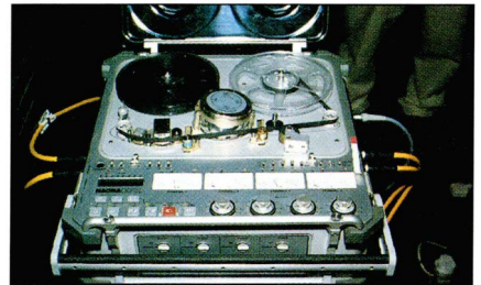
Serious kit: the Nagra D digital tape recorder used for the 96/24 location recording.
