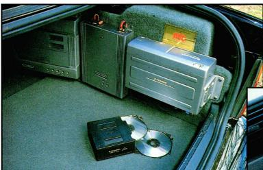
Power amps surround the *TS-W2RS* subwoofer while (right) the 12disc CD changer partially obscures the *RS-P1* processor at the heart of the ODR system.
