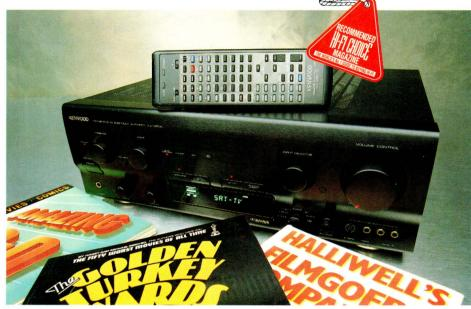
f soundfield features are a top priority then Kenwood's KA-V8500 AV amplifier is a purpose-built halfway house to Yamaha's DSP-A2070. In similar fashion, Kenwood employs a top-quality ADC to digitise incoming analogue signals before feeding samples to both a DSP (digital signal processor) soundfield synthesiser and digitally-steered SM5851 Pro-Logic chip.
