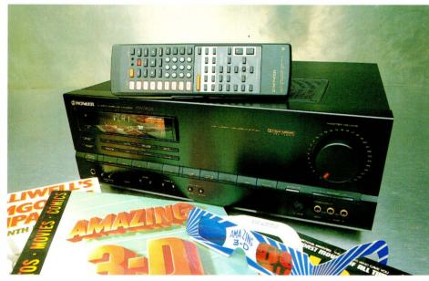
op of Pioneer's AV range, the VSA-D802S is the only one able to simulate Hall, Theatre, Jazz, Church and Dance soundfields using genuine DSP logic. This is as part of Yamaha's YSS215 AV processing circuit which includes a Pro-Logic decoder plus a 15-bit digital delay section that also adds extra reverb to the surround channel during DPL Theatre mode.
