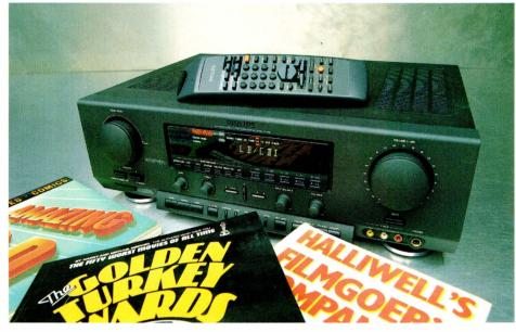
ith its latest 900 Series already brimming with DCC and CD players, digital loudspeakers and a digital tuner, you'd expect the complementary AV receiver to be similarly digital. In practice, only the FM/AM tuner section with its 30-presets, direct frequency access and station title memory has a digital heart.
