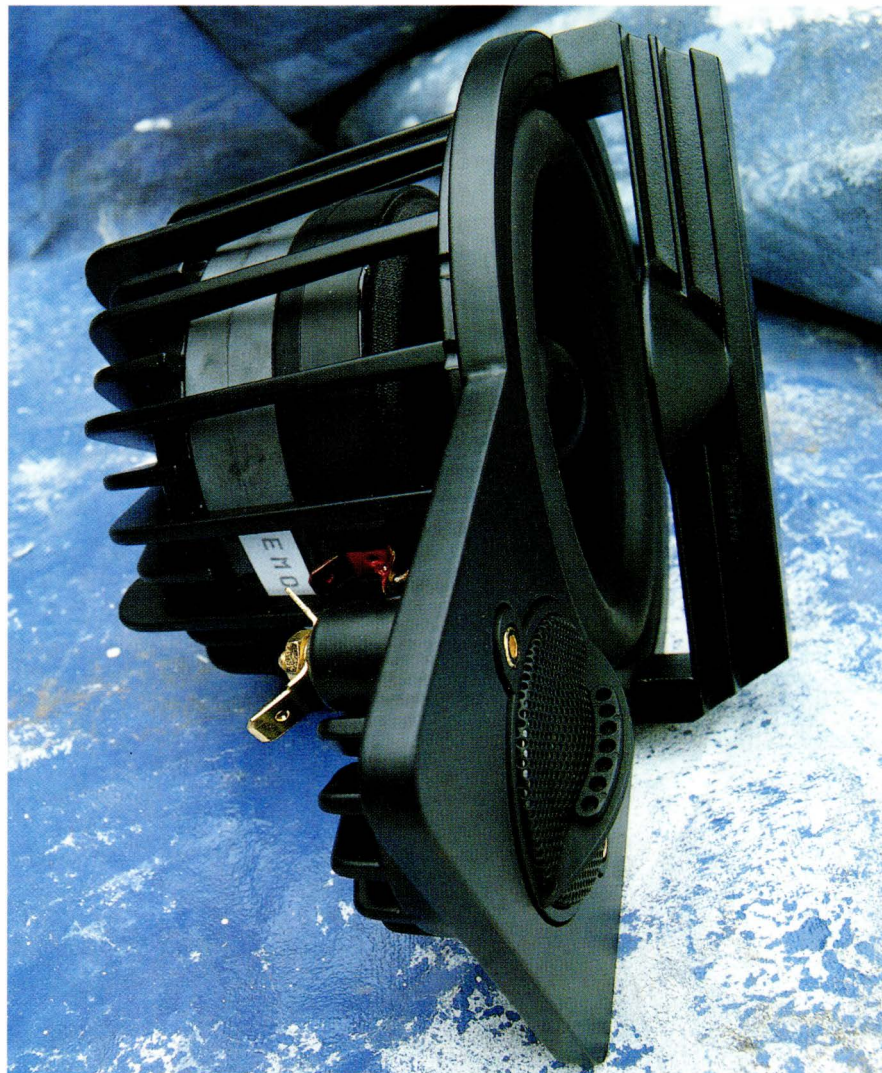
Bars over midrange and tweeter units (AMDs) absorb unwanted driver break up modes.
