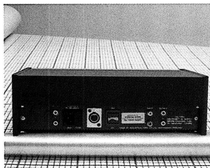
New IC, new wiring, new power supply, new everything... Avondale Audio's rebuilt Quad 405.
