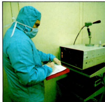
Optical centring of a stamper during the mechanical finishing stage (top), and the daily check on air cleanliness in the press shop.
