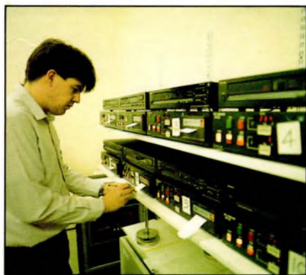
In the QA Section, discs are played on Toshiba CD players connected to 'CD checking' machines. Below, the steel-lined chamber used for the 'damp heat' environmental tests.
