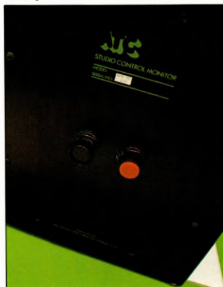
The formidable ATC SCM50. Crossover panel can be removed for active conversion, thus making it a SCM50A.
