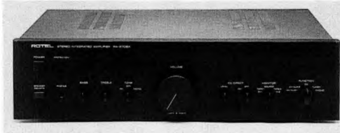
Rotel RA870BX: changing from 240V to 110V is a ten minute job for an engineer.
