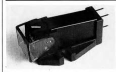
The 800MkII is clearly based on Ortofon's highly successful VMS series of cartridges, and appears to be most closely allied to the stalwart VMS10EII. The tubular alloy cantilever is fitted with an elliptical stylus at one end and a permeable armature at the other. This moves between coils set in the field of a permanent ring magnet – hence the term Variable Magnetic Shunt. The resulting output is extremely high at 6.5mV (5cm/sec peak) and so will drive any standard moving magnet input.
