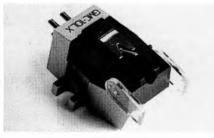
The GMC-10LX moving coil appears to share the same internal magnet assembly as the cheaper GMC-10EH, but far fewer turns on the armature places it firmly in the lowoutput class. Transient response should be improved by reducing the moving mass in this fashion, just as the fine line contact stylus bodes well for accurate groove tracing. Light to medium effective mass arms are best suited to this cartridge but, once again, the structural limitations of its plastic body cannot easily be overcome.
