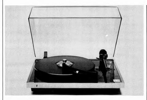
Townshend's new lower cost player retains the key Cranfield Institute of Technology derived features made familiar by the original *Rock*, including the radial silicone-filled trough which damps the arm/cartridge LF resonance by clamping the arm solid at low frequencies using an outrigger attached to the headshell. Various arms can be specified, but for this test the *Avalon* was fitted with a Rega *RB250*.
