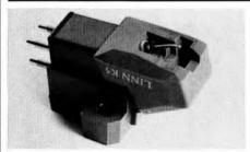
The K5 is cheapest of Linn's K-series and appears to adopt the dual-magnet generator system used by Audio Technica in its cheaper MM cartridges. Indeed, both the elliptical stylus, crimped alloy cantilever and compliant damper are very similar to those employed in the AT-420E. Nevertheless, because of the K5's lower bodyweight, its mean 14cu compliance makes it better suited to medium mass tonearms.
