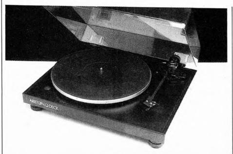
The *Q-Deck* is designed to meet the non-specialist user at least half way. The player works almost straight from the box. There's no suspension to adjust; the arm is non-interchangeable; and an Ortofon *OM10* cartridge is supplied fitted. Speed change is by a discreet dome switch, the motor being driven by a simple L-C oscillator.
