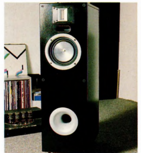
Townshend Glastonbury uses a metal-coned Jordan driver, reflex port, and 'brute force' technique of plaster and steel to achieve cabinet rigidity.
