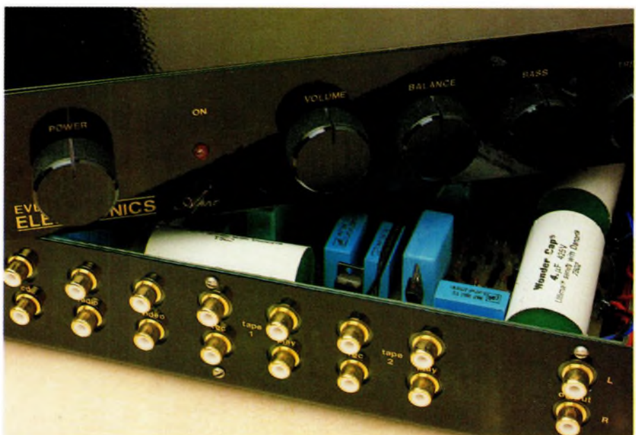
Back to front, the gold-plated socketry of the Apex 'S' series pre-amp.
