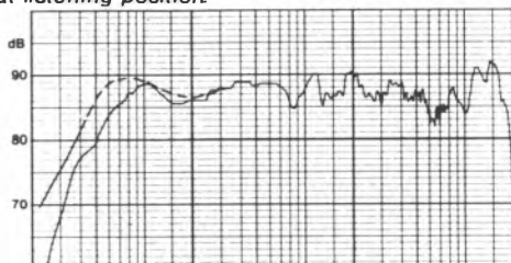
Reference sinewave response (1m on axis, 2.83V input shows sensitivity) (dashing corrects for chamber LF, dotting shows response without grille).
