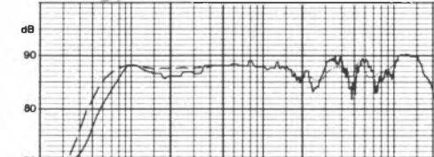
Reference sinewave response (1m on axis, 2.83V input shows sensitivity) (dashing corrects for chamber LF, dotting shows response without grille).
