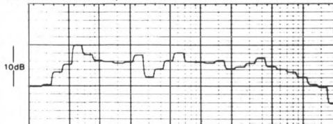
Averaged forward characteristic response in room at listening position.
