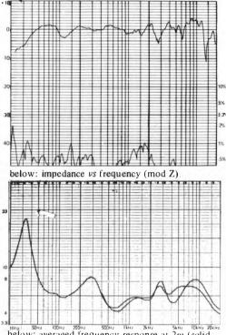
below: averaged frequency response at 2m (solid curve on axis, dotted curve 10° vertical dashed curves 30° horizontal L&R) vertical scale 1dB/div.
