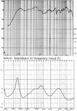
below: averaged frequency response at 2m (solid curve on axis, dotted curve 10° vertical, dashed curve 30° horizontal) vertical scale 1dB/div.
