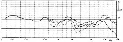
$^{1_3}$ -octave averaged frequency response, 2m solid axial; dotted 10° above and below; dashed 30° horizontal 79
