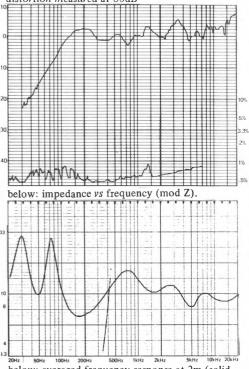
below: averaged frequency response at 2m (solid curve on axis, dotted curve  $10^{\circ}$  vertical, dashed curve  $30^{\circ}$  horizontal) vertical scale 1dB/div.
