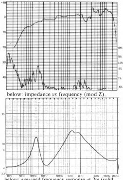
below: averaged frequency response at 2m (solid curve on axis, dotted curve 10<sup>0</sup> vertical dashed curves 30<sup>0</sup> horizontal L&R) vertical scale 1dB/div.
