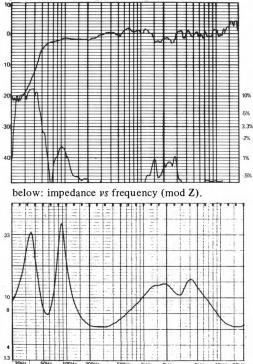
below: averaged frequency response at 2m (solid curve on axis, dotted curve 10<sup>o</sup> vertical, dashed curve 30<sup>o</sup> horizontal) vertical scale 1dB/div.
