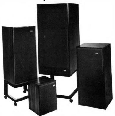
BCI A standard monitor loudspeaker in sound broadcasting studios throughout the U.K.; also used in recording studios where the requirement is for accurate reproduction rather than an "impressive" sound. The BCI is a three-unit bass reflex design using a Spendor 200mm cone driver for bass/midrange, Power handling is 55W.
