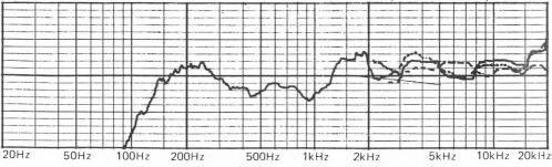
When a test record is cut, a tiny amount of wow and flutter creeps into it from the wow and flutter of the cutting machine
