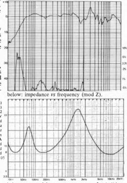
below: averaged frequency response at 2m (solid curve on axis, dotted curve  $10^{\circ}$  vertical, dashed curve  $30^{\circ}$  horizontal) vertical scale 1dB/div.
