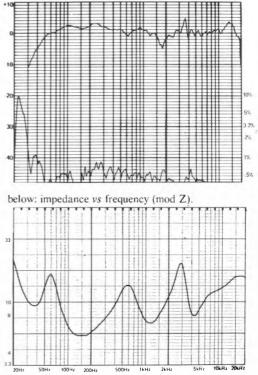
below: averaged frequency response at 2m (solid curve on axis, dotted curve  $10^{\circ}$  vertical, dashed curve  $30^{\circ}$  horizontal) vertical scale IdB/div.
