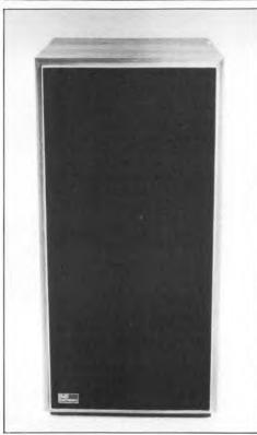
The Mark I version of this speaker was included in the previous *Hi-Fi Choice Loudspeakers*, the *TLS80* being a large, free-standing enclosure of imposing dimensions. A purpose built steel stand with an inbuilt angle of tilt is supplied with the speakers, which come in left/right mirror pairs and are provided with a switched HF control allowing nominal degrees of lift or cut to suit room acoustics and position.
