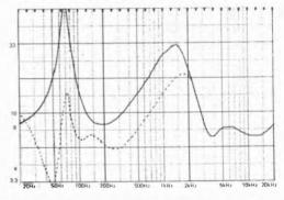
below: averaged frequency response at 2m (solid curve on axis, dotted curve 10° vertical, dashed curve 30°-horiztontal) vertical scale 1dB/div.
