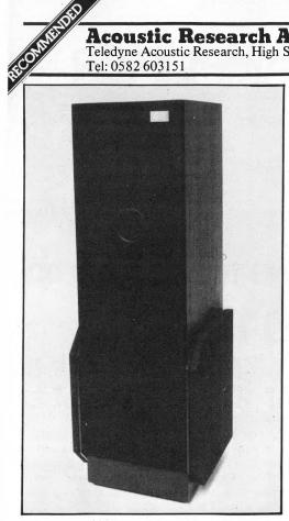
Similar to the larger AR9, the 90 makes a small concession in ultimate power handling and bass extension by allowing the use of two 250mm low frequency drivers per enclosure instead of the 300mm units used for the'9s. The remaining drivers are the same, namely a 200m pulp cone midrange a 38mm soft dome lower treble, and a 19mm soft dome upper treble, arranged in a vertical-in-line format. An 'acoustic blanket' (a thick felt layer) surrounds the drivers.
