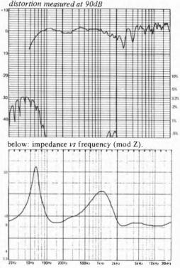
below: averaged frequency response at 2m (solid curve on axis, dotted curve 10<sup>o</sup> vertical, dashed curve 30<sup>o</sup> horizontal) vertical scale 1dB/div.
