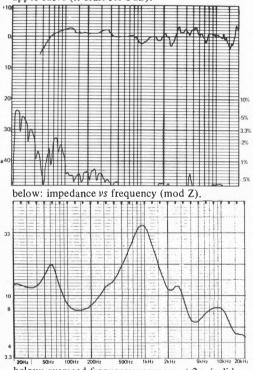
below: averaged frequency response at 2m (solid curve on axis, dotted curve 10° vertical, dashed curve 30° horizontal) vertical scale 1dB/div.
