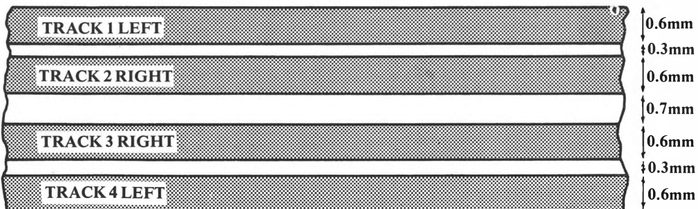
Typical track dimensions for domestic use in cassettes
