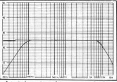
A typical pen chart of the tone controls with rumble filter.
