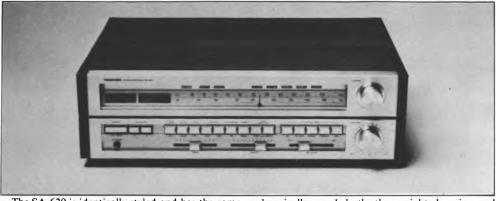
The SA-620 is identically styled and has the same facilities throughout as the model SA-520, with the exception that two extra push buttons (false teeth) are provided for audio muting and tone control cancelling. On the back panel, unlike the SA-520, break points are mounted to enable external equipment to be inserted inbetween the pre-amplifier and power amplifier sections. The maximum power output though is somewhat higher, 71W into 8 ohms, rising to 105 watts into 4 ohms.
