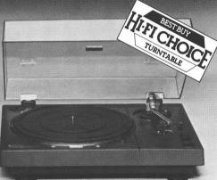
Stereo turntable is designed to meet the extra demands at the top end of the Hi-Fi range. The direct driven platter is operated by a brushless DC motor to minimise speed loss or fluctuations. Controls include:- recessed stroboscope and 'plus' and 'minus' fine speed adjusters. Wow and flutter is less than 0.04% WRMS.
