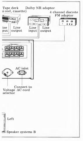
Some receivers can be interconnected with three pairs of speakers, but usually their instruction manuals indicate that not more than two pairs should be connected at any one time. Although most receivers are protected against too great a current requirement from the speaker systems, some do not have this protection, and so if you demand too much of the amplifier you run the risk of blowing up the output stage. I therefore strongly advise you to read the instruction manual.
