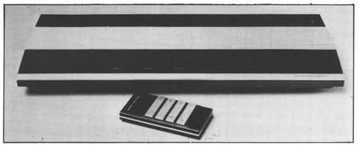
This remarkable receiver with a remote control facility contains some very unusual features. In particular, the volume control is touch operated with internal circuitry automatically altering volume, either on the set itself or by remote control. The volume unfortunately continues to alter for a second or so after pressure is released, and so a panic mute button is provided!
