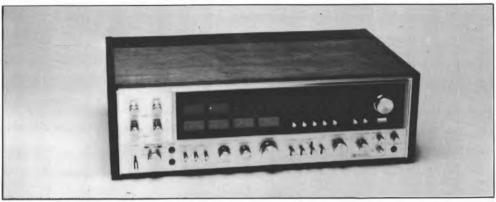
The UK version of this model incorporates a modification which uses one of the two tape replay monitors for Matrix H decoding. Incorporating four output amplifiers and with the provision of driving two four-channel systems, it can decode CD4, SQ, and QS discs, the last also being used when matrix H is switched in. The four amplifiers can be switched to give higher power for stereo, but normally gives 100W per channel into 8 ohms, but only 70W continuous into 4 ohms.
