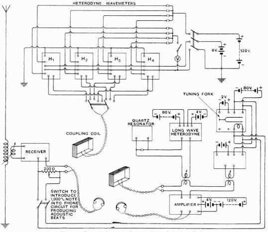
Fig. 1.—General diagram of connections of the installation.
