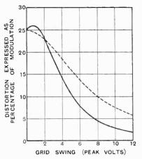
Fig. 14.—Showing reduction of distortion with increasing grid swing, grid bias 12 volts. The full curve shows the actual distortion; the dotted curve is the distortion calculated for a hyperbolic rectification curve (see Figs. 9 and 10).
