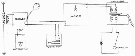
Fig. 8.—Diagram of connections of the apparatus for recording scintillation (frequency modulation).
