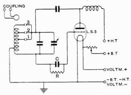
Fig. 2.—Diagram of connections of the heterodyne wavemeter.
