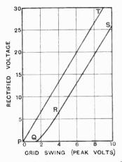
Fig. 15.—Rectification curves corresponding to ideal characteristic of Fig. 7. PT is drawn for the correct grid bias of 12½ volts (B, Fig. 7), PQRS for a grid bias of 14 volts. If the grid swing exceeds 4 volts in the latter case, the distortion is small. With a grid swing of 1½ volts the distortion is great. When the grid bias is correctly adjusted rectification is distortionless for all values of the grid swing.
