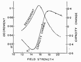
Fig. 2. — Experimental. a. Field strength at which the electron frequency = field frequency. b. Decrement for cold cathode.
