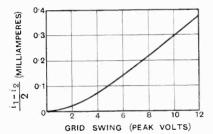
Fig. 13.—Curve deduced from Fig. 12 in the manner indicated in Fig. 11 ((a) and (b)). Grid bias 12 volts.
