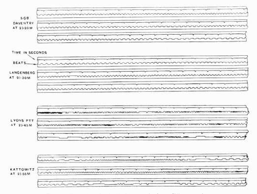
Fig. 9.—Examples of scintillation records for 4 different stations.
