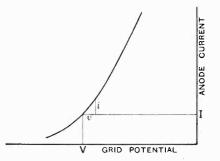
Fig. 2a.—Relation between grid potential and anode current.
