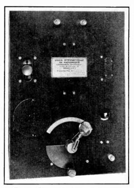
Fig. 3.—Photograph of wavemeter panel.
