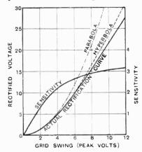
Fig. 9.—Rectification curve for PM3 valve, R = 130,000 ohms, voltage about 190. The parabola most closely approximating to the curve for small values of the grid swing is also shown. The general features of the curve are more nearly those of an hyperbola, which is also shown. It is seen that for small grid swings the sensitivity is practically proportional to the swing. As the swing increases, however, the sensitivity approaches a limiting value.
