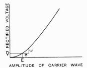
Fig. 3a.—Relation between rectified voltage and amplitude of carrier wave.
