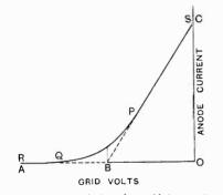
Fig. 8.—Characteristic of rectifying valve. It is seen that as grid swing increases the effective deviation from the ideal A B C diminishes.
