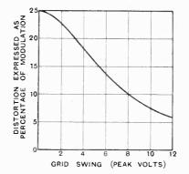
Fig. 10.—Showing reduction of distortion with increasing grid swing—hyperbolic rectification curve (see Fig. 9).
