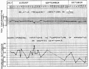
Fig. 5.—Curves showing the variations in calibration of Range 2 of the heterodyne wavemeter No. 2, for a frequency of 966 kilohertz and variations in temperature.
