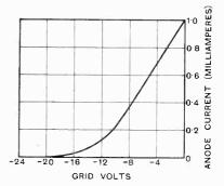
Fig. 12.—Characteristic for PM3 with anode resistance of 130,000 ohms.
