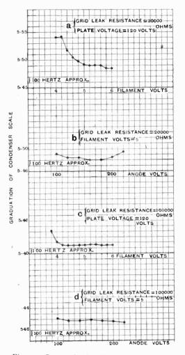
Fig. 4.—Curves showing the variation of calibration of the heterodyne wavemeter as a function of low-tension and high-tension voltages for a grid leak resistance of 20,000 ohms and 100,000 ohms.
