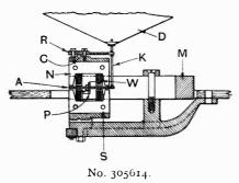
reed R having a very high natural period of vibration, preferably exceeding 10,000 cycles per second. The reed is forced by two screws against a rod Cresting in a groove or notch formed in a rigid part of the mounting, this arrangement allowing the reed to be correctly centred. The loud speaker diaphragm D is mounted on the rod K at a point
