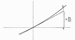
Fig. 6.—For small values of x the tangent is a sufficient approximation to the curve and y may be assumed equal to  $x \frac{dy}{dx}$ . As x increases it becomes necessary to allow for the fact that  $\frac{dy}{dx}$  is changing.
