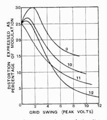
Fig. 16.—Showing variation of the distortion characteristic with the grid bias. The corresponding grid bias (in volts) is indicated on each curve.
