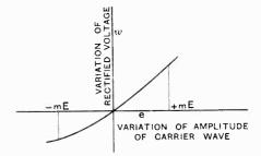
Fig. 3b.—Relation between changes in amplitude of carrier wave and variation of rectified voltage.
