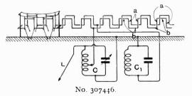
of half the working wavelength. Finally the length of each horizontal is chosen so that the induced currents in each of the verticals are in phase. The centre of the aerial system as a whole is earthed through a tuned loop circuit C, the reflector system being similarly grounded through a tuned circuit  $C_1$ .
