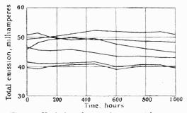
Fig 3.—Variation of saturation current from an oxide-coated cathode made by the barium vapour process with life. Total emission of Mullard PM5 filament operated at 5.5 volts. Grid anode potential 80 volts. Grid connected to anode.
