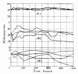
Fig. 2.—Variation of saturation current from various oxide-coated cathodes with life.
