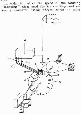
separate sets of spirally-staggered holes a, b, c are used to analyse simultaneously three distinct segments 1, 2, 3 of the object being televised. The elative setting of the spiral series of holes a is such
