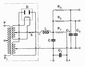
where the circuit is designed to pass the considerable output required for power amplification. Resistance-capacity networks have been used as an alternative, the smoothing action in this case increasing as the product of the resistance and capacity elements in circuit. The latter method has, however, the drawback of introducing a large voltage drop, which, particularly in the first stage, varies according to the current consumption of the latter or power amplifying stages.
